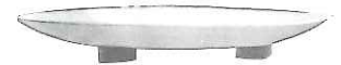
Large flat pieces may be placed on kiln's floor if short posts are used to allow heat circulation.
