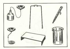
The density of solid bodies and liquids can be determined simply and reliably with the Density Determination Kit (Optional accessory).
