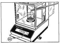
When weighing in finely to approach the target weight, the last digit automatically reappears:
