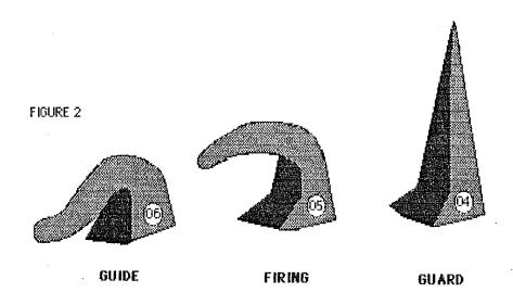
After making your initial performance check, we recommend you test fire approximately every 25 firings including a set of cones of the same numbers in your firing and placing it on the same shelf and in the same general area each time and firing to the specifications above. Save these cones as records of the firing. Place them in a row on a shelf near your kiln and review them periodically to note variations or drift in successive firings.
