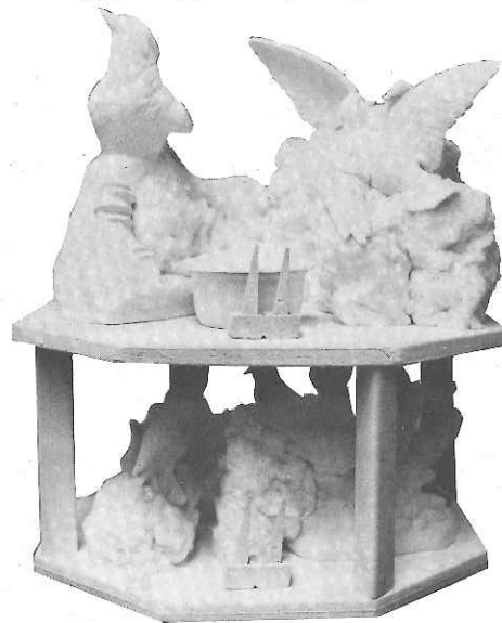
Porcelain greenware is placed directly on the kiln washed shelves or brick bottom and supported by ceramic fiber. Note that pieces to be used together must be fired together, such as the box with lid on the top shelf. Two, large cones should be located behind each peephole.
