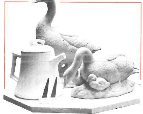
Small, light pieces of greenware can be placed directly on the brick bottom
