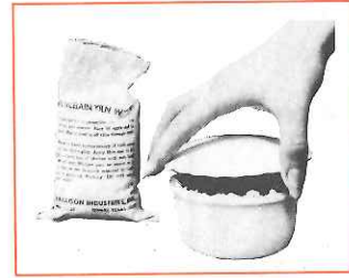
Dry, all-purpose, high fire, kiln wash is used to prevent lid from sticking to box.
